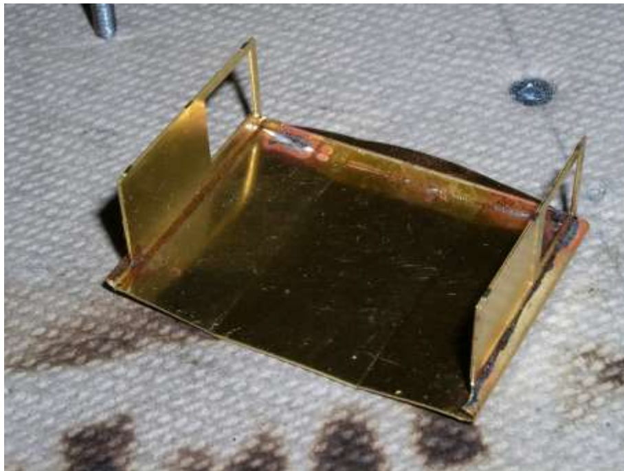
Figure 024 showing the doors soldered in place on solid end.
