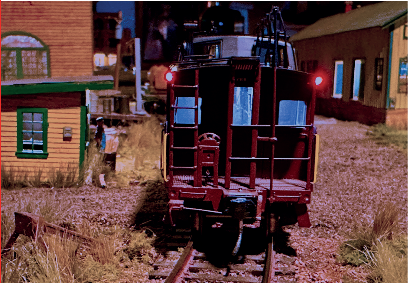
Fiber optics make good marker light lenses. This PRR caboose uses them underneath the roof of the rear platform. It's an attractive detail.
